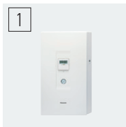
1 High Efficiency Aquarea Hydrokit New indoor unit design. New A-class pump with 7 speeds, expansion vessel of 10L and selectable back-up heater (3/6/9kW).
